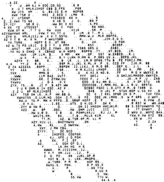
Figure 1. Example of a part of an infinite cluster grown at criticality. The asterisk '*' is an arbitrary point in the cluster. Sites belonging to shells of successive chemical distance are designated by successive letters of the alphabet (starting with 'B'), and dots designate sites which were tested and found to be empty. The cluster was generated on a triangular lattice, obtained by taking points to lie on a square lattice and regarding sites along one of the diagonal directions as nearest neighbours.
